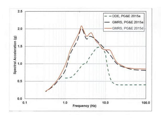
Figure 3.5-1. Initial Ground Motion Response Spectrum (GMRS; black dashed line) and Double Design Earthquake (i.e., SSE; green dashed line) from SHSR for DCPP (PG&E, 2015a). Revised GMRS (red solid line) from PG&E (2015d).
