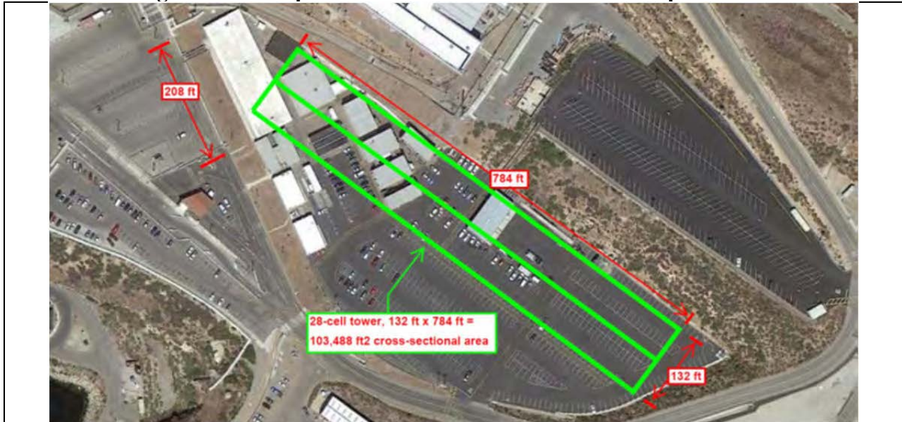
Figure 9. 28-cell Unit 2 cooling tower using cell dimensions of 66 feet width by 48 feet length to achieve performance similar to SPX basecase specification
