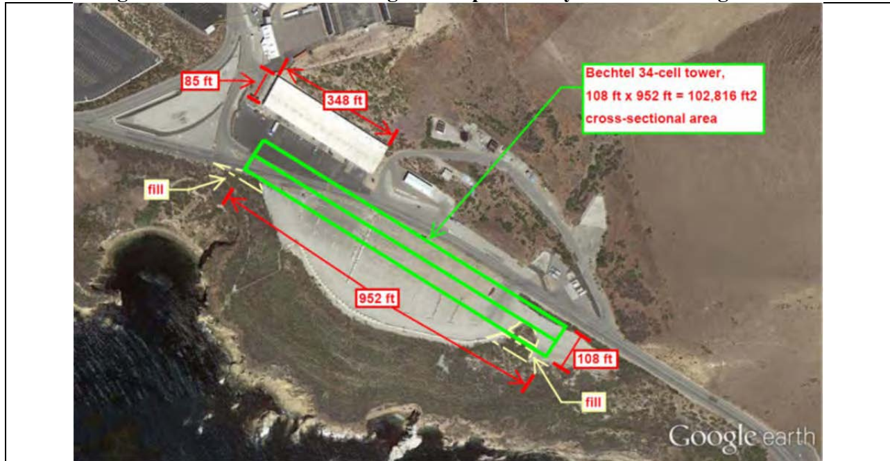
Figure 11. 34-cell Unit 2 cooling tower specified by SPX in Parking Lot 1 56
