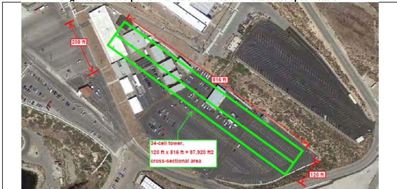
Figure 8. 34-cell Unit 2 cooling tower using cell width of 60 feet per Bechtel and 48 feet length to achieve performance similar to SPX basecase specification
