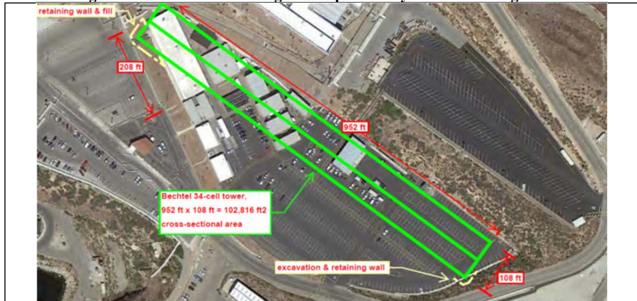
Figure 6. 34-cell Unit 2 cooling tower specified by SPX in Parking Lot 7 45
