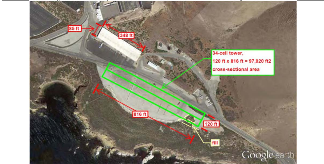
Figure 12. 34-cell Unit 1 cooling tower using cell width of 60 feet per Bechtel and 48 feet length to achieve performance similar to SPX basecase specification
