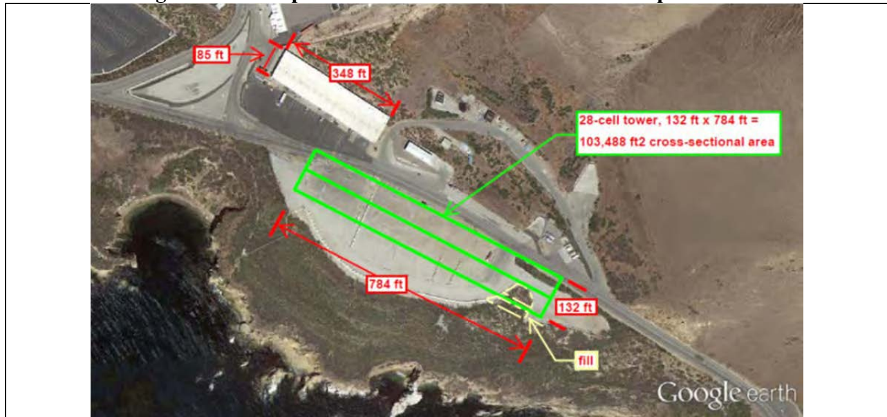
Figure 13. 28-cell Unit 2 cooling tower using cell dimensions of 66 feet width by 48 feet length to achieve performance similar to SPX basecase specification
